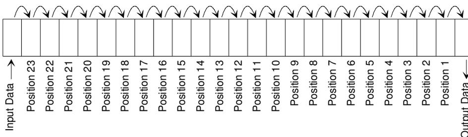
This type of data manipulation is called a data shift register. With each input pulse, data is shifted one position in the array (or sequential group of registers).
